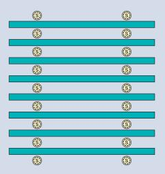
IF GAP BETWEEN TOP OF RACK AND CEILING IS LESS THAN 300mm THEN TREAT AS WALL AND PROVIDE DETECTION IN EACH AISLE
