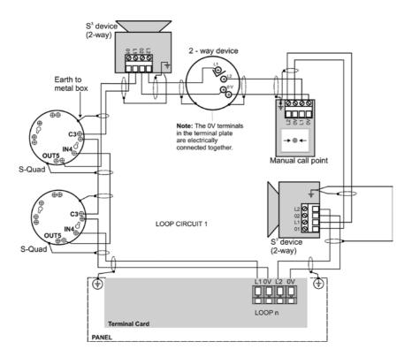
Each loop circuit can accept connection of up to a maximum of 200\* addressable devices per loop. To maintain earth continuity on a loop it is important for the loop cable screen to be continued through each system device, whether the earth is connected to a device or not.
