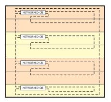
Example of a networked fire alarm in a multi-storey building, showing standard cable grade throughout provided that there is diverse routing of the network cable loop.
