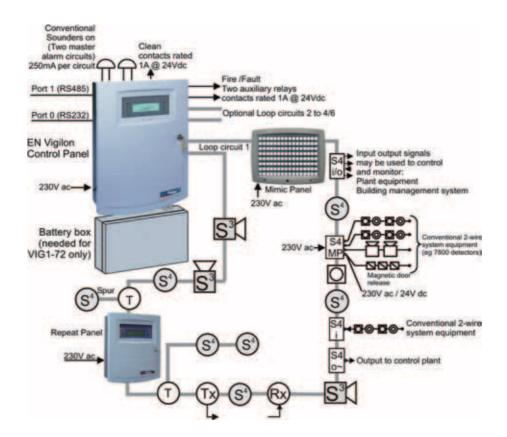
Please note that a Vigilon loop can accept upto 200 devices, the Nano single loop panel supports 127 devices.
