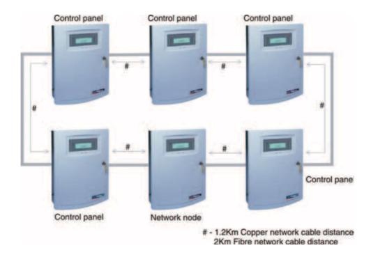
Upto 31 Vigilon / Vigilon Compact panels can be connected to a network in the form of a secure loop using the cables detailed. Larger network capacity can be accommodated, please contact Gent by Honeywell for further support and details
