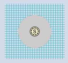
WHERE AIR IS FORCED THROUGH A PERFORATED CEILING, THE DETECTOR SHOULD BE MOUNTED ON A SOLID BAFFLE WITH A MINIMUM DIAMETER OF 1200mm
