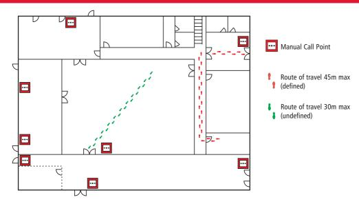
Note: In order to comply with the requirements of Building Regulations Approved Document Part M, which requires electrical switches including manual call points (MCPs) to be mounted at between 1M + or - 200mm on wheel chair access routes, these should be listed as a Variation on the certificate as BS requires MCPs to be mounted at 1.4M + or - 200mm.
