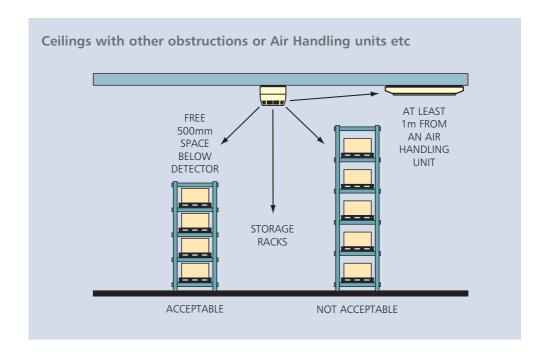
One of the most common mistakes is to mount a smoke sensor adjacent to the air conditioning intake or outlet grill. The minimum distance between the two should be at least 1 metre and further if possible. This is due to the fact that smoke may have difficulty penetrating the sensor when the air conditioning is switched on. Also there is a greater risk of the sensor becoming contaminated and giving rise to false alarms.
