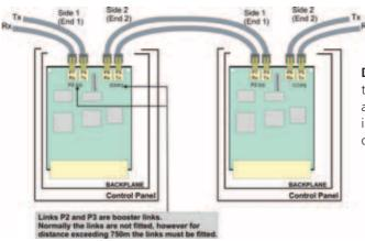
**DO NOT** mix cables of different types on the same network, as this will create impedance imbalance and disruption to data communication.
